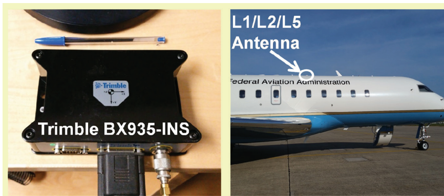
FIGURE 1 A GNSS receiver and antenna used on FAA Global 5000 business jet.
