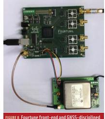
FIGURE 8 Fourtune front-end and GNSS-disciplined reference oscillator
