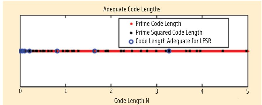
FIGURE 1 Adequate code lengths for LFSR-based sequences, prime, and prime-squared length sequences
