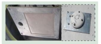
FIGURE 5 Antennas: LHCP antenna (left) and RHCP antenna (right)
