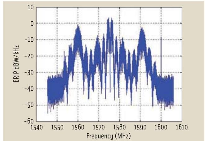
FIGURE 2 L1 CBOC interplex spectrum
