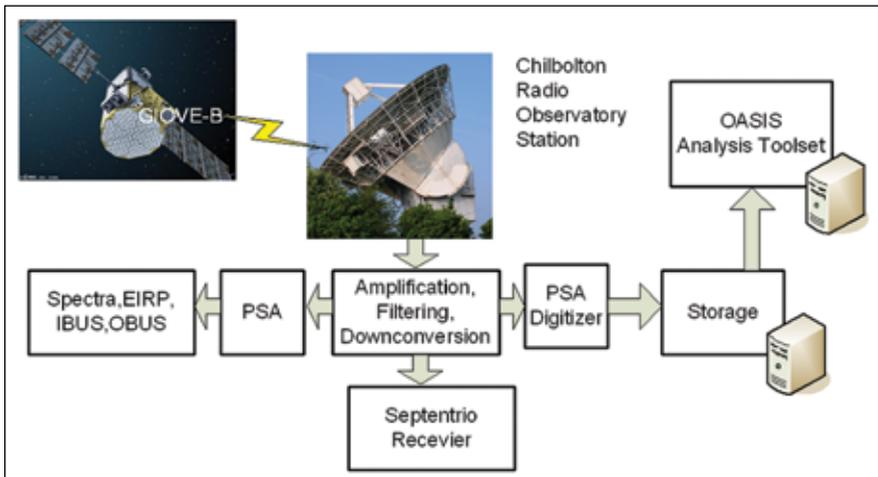
**FIGURE 1** System for acquisition and analysis of GIOVE-B navigation signals at in-orbit test station, Chilbolton, UK
