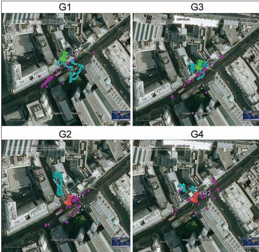
**FIGURE 17** The positioning solution shown in satellite image view (blue dots represent locations of the conventional GNSS solution; purple dots denote positioning solutions provided by the new system; the pushpin tags represent the true location of the site in each case; Image © 2013 Bluesky)
