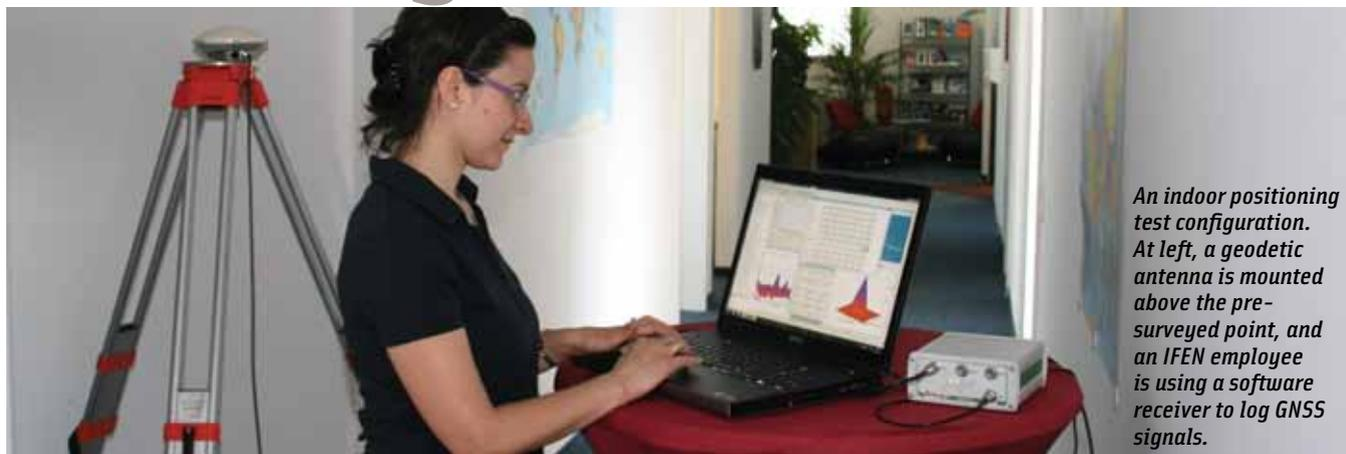
*An indoor positioning test configuration. At left, a geodetic antenna is mounted above the pre-surveyed point, and an IFEN employee is using a software receiver to log GNSS signals.*
