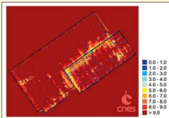
FIGURE 6 Average number of available AGNSS signals in acquisition mode
