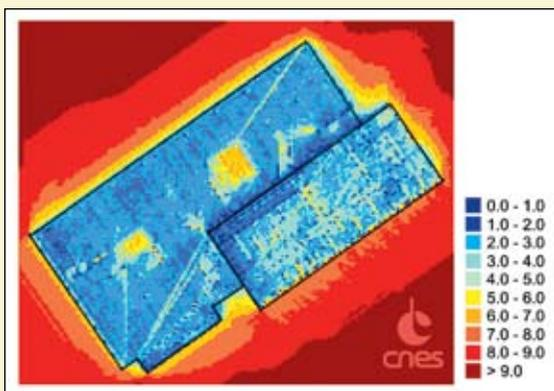
FIGURE 3 Average number of available GPS signals in acquisition mode
