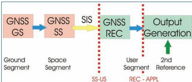
FIGURE 4 Flow of information and signals between a GNSS Ground Segment (GS) and Space Segment (SS), through the Signals in Space (SIS) to the Receiver (REC) and the final output of the application (APPL).
