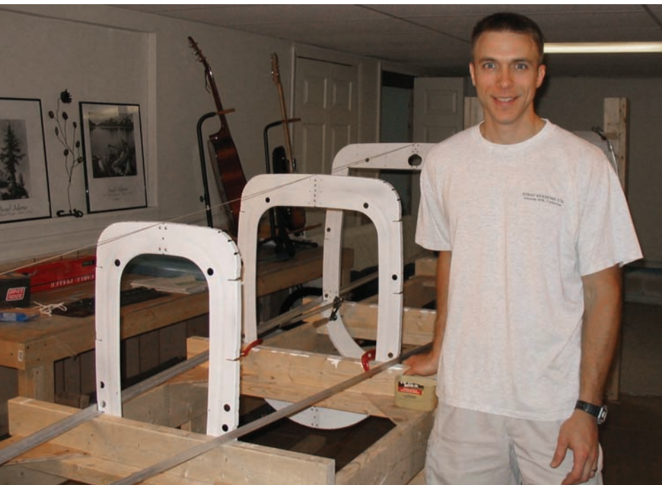
Veth proudly poses with his RV-8A fuselage components securely fastened in a jig. The RV-8A is a two-place, tandem, experimental aircraft that is home-built from kit components. When completed, he plans to use the aircraft as an experimental navigation testbed.
