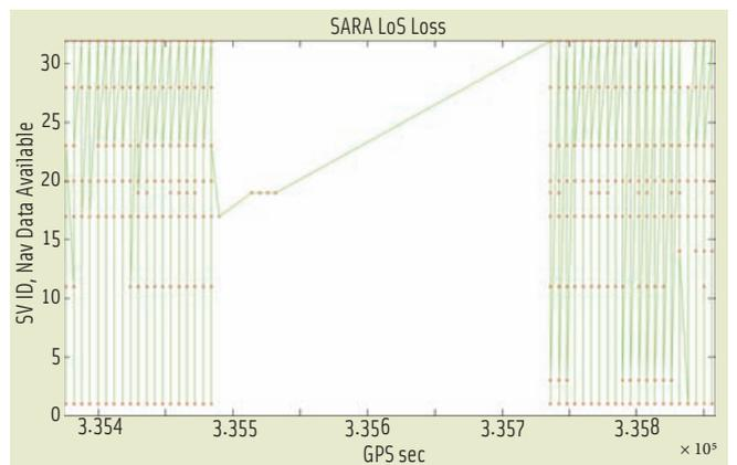
FIGURE 19 Frame data evolution by PRN code during an LoS loss event.
