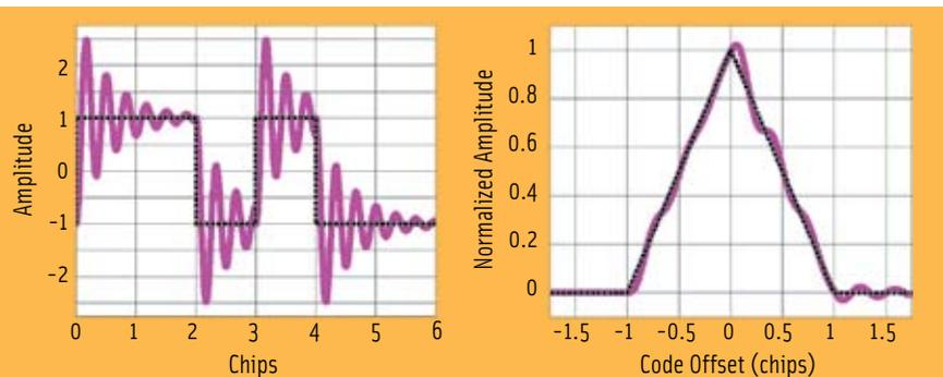
**FIGURE 5** Example of analog code distortion model and its effect on the correlation peak
