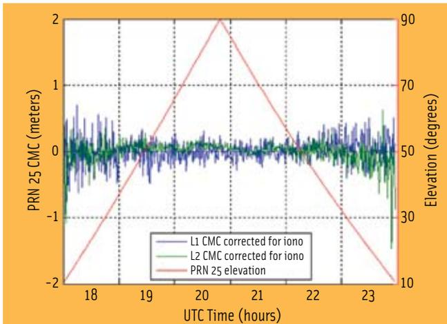
**FIGURE 3** SVN 62 code-minus-carrier measurements after applying a dual-frequency ionosphere correction. The clock, orbit, troposphere, and ionosphere errors are all eliminated. No apparent elevation-dependent bias exists in either L1 or L2 measurements.
