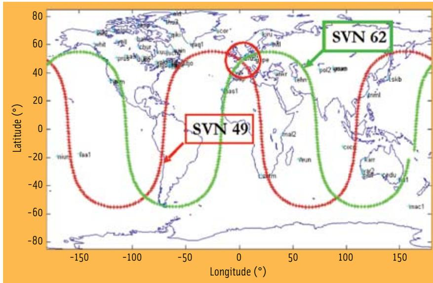
FIGURE 1 Ground tracks of SVN 49 and SVN 62. The receivers shown on this map are the 69 out of 300+ IGS sites that output both SVN 49 and SVN 62 measurements as of Day 170, Year 2010.
