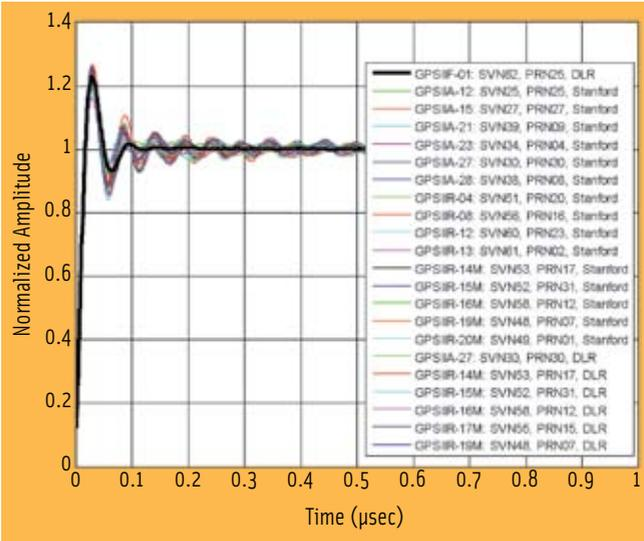
FIGURE 8 Comparison of the step responses on the L1 C/A codes of 17 GPS satellites. The response of SVN62 is depicted by the heavy black trace.
