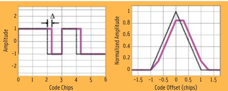
**FIGURE 4** Example of digital code distortion model and its effect on the correlation peak
