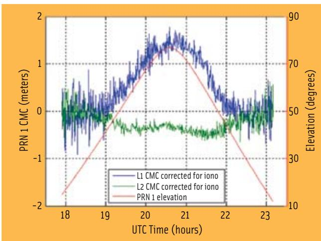
FIGURE 2 SVN 49 code-minus-carrier measurements after applying a dual-frequency ionosphere correction. The clock, orbit, troposphere, and ionosphere errors are all eliminated. An obvious positive elevation-dependent bias exists in the L1 C/A measurements. A slight negative elevation-dependent bias is seen in the L2 measurements.
