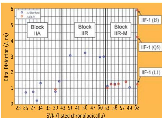
FIGURE 7 Recent digital distortion summary plotted as a function of SVN (from earliest to latest launch date). This uses data taken between June 2008 and 2010. Three results appear for SVN 62 signals: one each for L1 C/A code, I5 (L5, In-phase), and Q5 (L5, quadrature).
