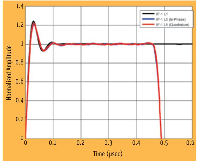
FIGURE 9 Comparison of the step responses on three codes transmitted from SVN 62: L1 C/A (black), L5 in-phase (blue) and quadrature (red).
