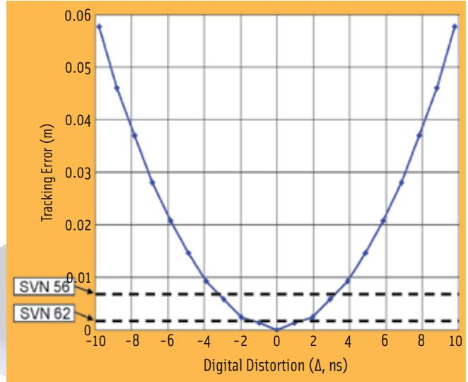
FIGURE 10 Modeled WAAS user tracking errors on L1 C/A code due to digital distortion only. Errors have been differentially corrected by the WAAS reference station receiver (Early-minus-late discriminator at 0.1-chip spacing and a filter having 18MHz bandwidth). User receiver properties are modeled according to the constraints defined in the Minimum Operational Performance Standards (MOPS) DO-229D (RTCA, Inc.).
