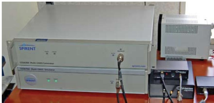
FIGURE 1 Single- and multi-channel simulators, GPS/Galileo (on top) and GPS/GLONASS software receiver USB front end with controlled power source
