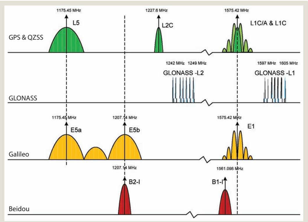
FIGURE 2 The spectrum of existing civil signals
