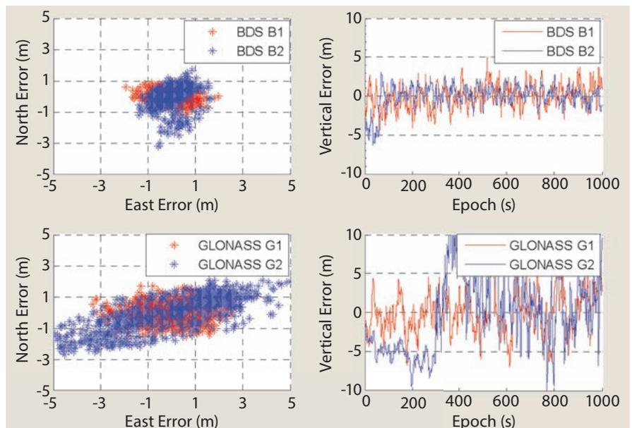
FIGURE 20 Positioning results of BDS and GLONASS signals
