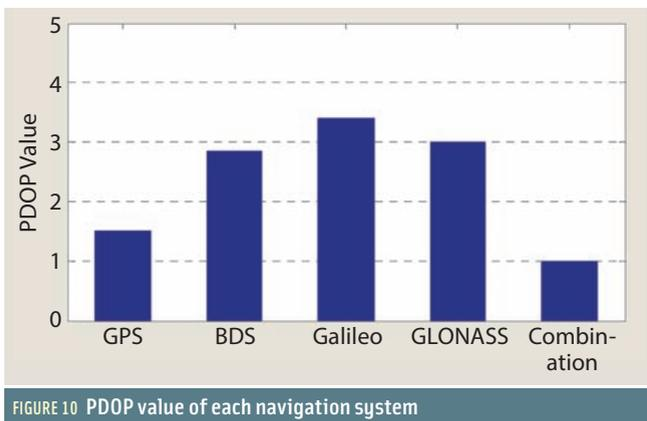
FIGURE 10 PDOP value of each navigation system
