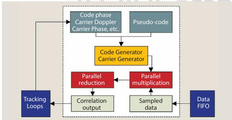
FIGURE 7 GPU-based correlator
