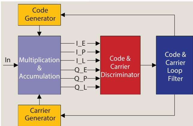
FIGURE 6 Code and carrier tracking loops
