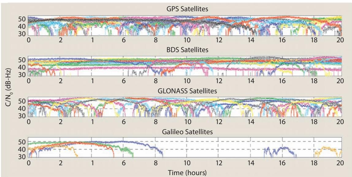
FIGURE 21 Satellite carrier-to-noise ratios during monitoring of four GNSS systems
