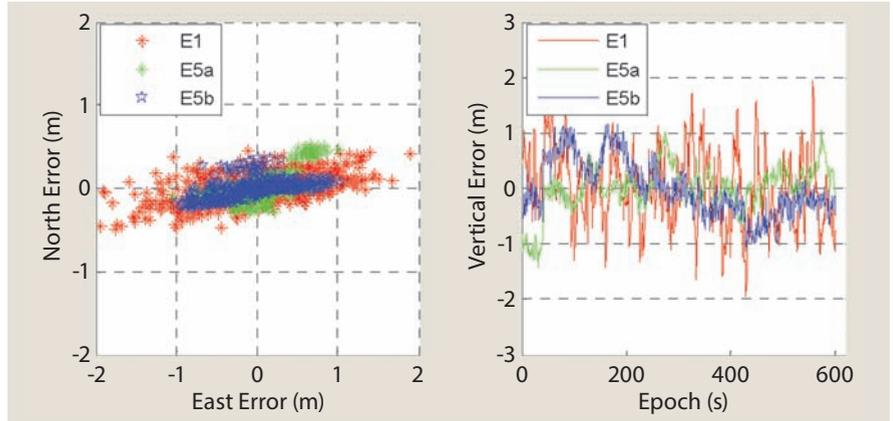
FIGURE 13 Positioning results of GALILEO signals
