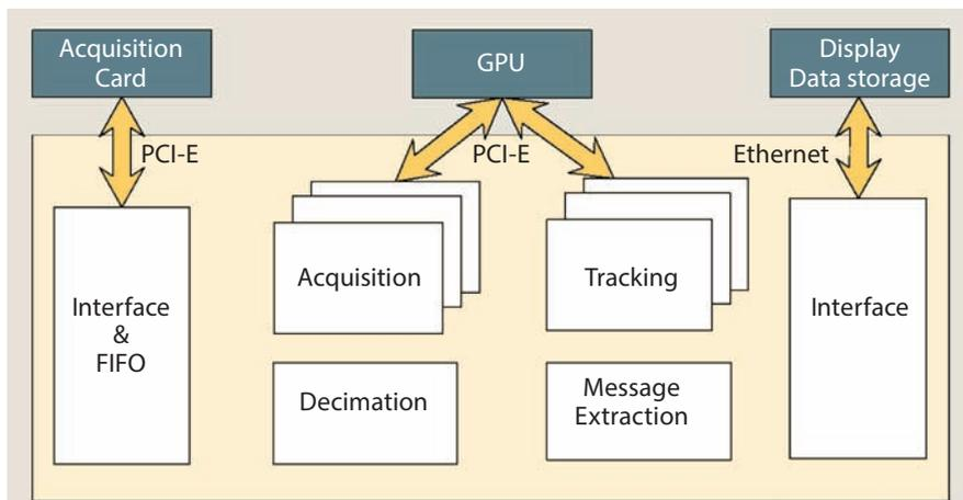
FIGURE 4 Software architecture in PC
