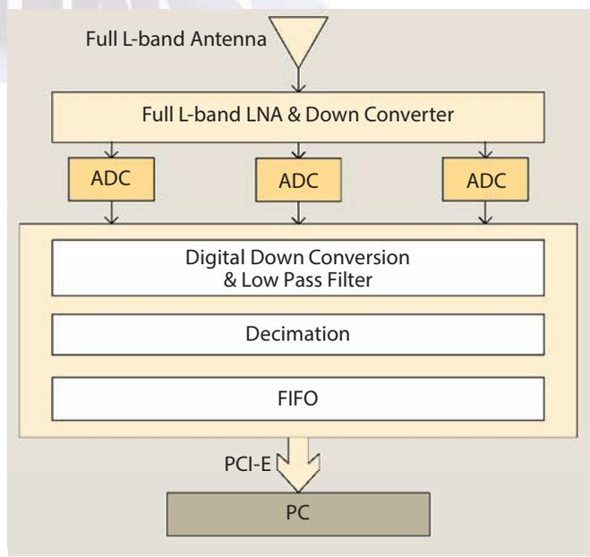
FIGURE 3 STARx front-end and data acquisition card
