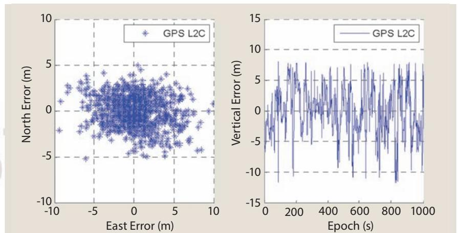
FIGURE 19 Positioning results of L2C signal
