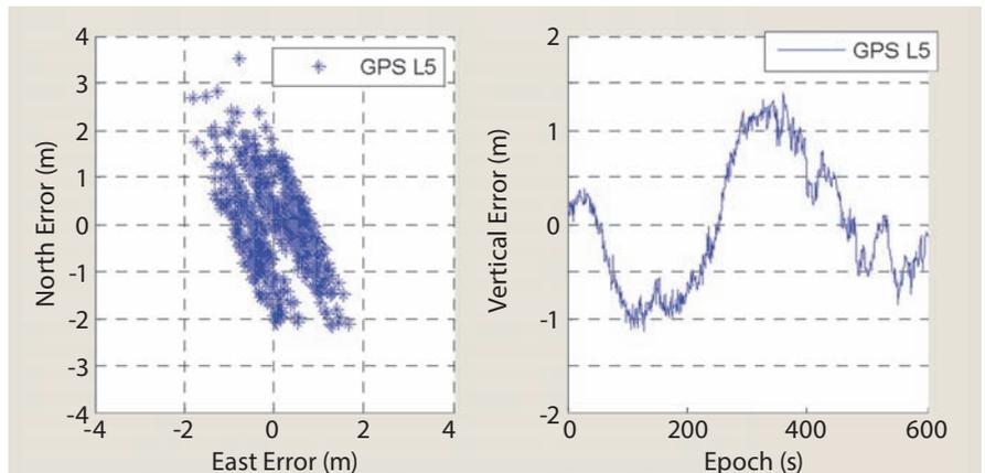
FIGURE 16 Positioning results of L5 signal
