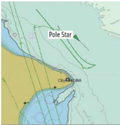
FIGURE 3 Extract of a vessel traffic image during the jamming trial. GPS jamming resulted in erroneous positions being reported for the trial vessel "Pole Star," giving the impression that she has sailed across the peninsula.
