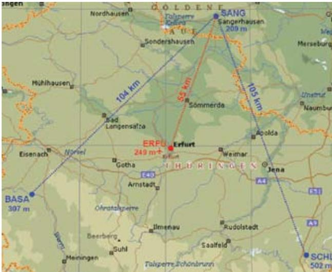
FIGURE 5 Type “Thinned Out”: A slightly sparser network triangle with a baseline length of 55 kilometers to the nearest reference site.
