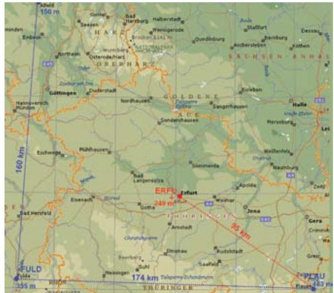
FIGURE 6 Type “Challenging”: Network triangle configuration with a baseline length of 95 kilometers to the nearest reference station.
