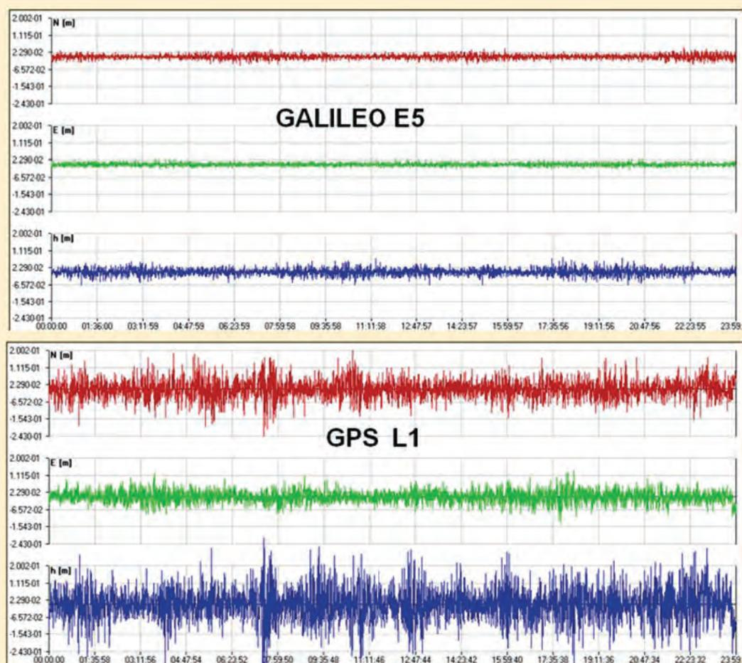
FIGURE 5 Comparison of the time series of the three coordinate components using simulated Galileo E5 (upper plot) and GPS L1 (lower plot) CPC results; 2.290-02 is read 2.290·10<sup>-2</sup> meters; GNSS time of day format is hh:mm:ss
