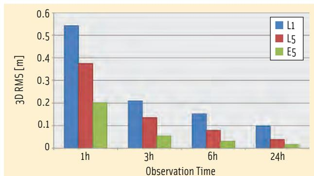
**FIGURE 9** Comparison of the 3D RMS error of different time series using Galileo E5, GPS L1 and GPS L5 CPC results
