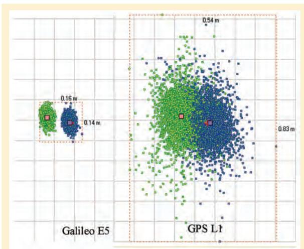
FIGURE 7 Results of the positions comparison for two different periods of observation using single-frequency data
