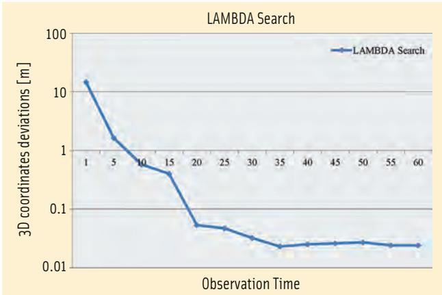
FIGURE 11 3D coordinate deviations in Galileo E5 single-frequency positioning by using LAMBDA search to solve the ambiguity term
