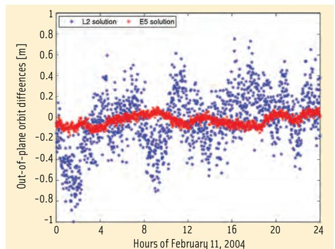
FIGURE 17 Out-of-plane orbit differences of kinematic orbit solutions from L2 and E5 with respect to ENVISAT reference orbit, February 11, 2004
