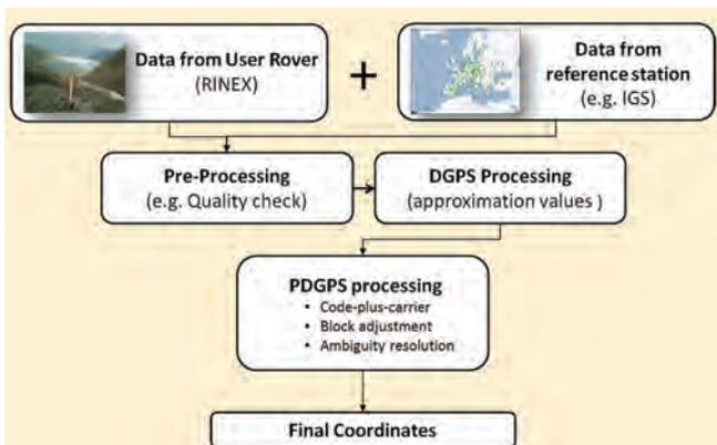
FIGURE 4 Processing procedures of Galileo E5 single-frequency data
