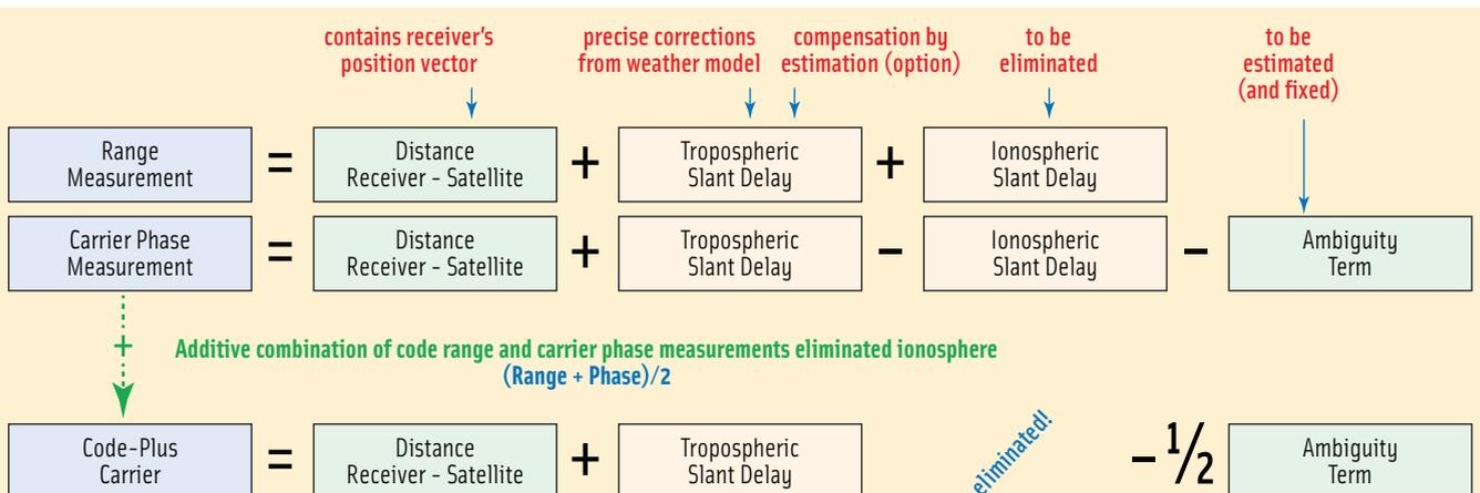
FIGURE 3 Simplified observation equations of single-frequency range and phase measurements by addition of both observables
