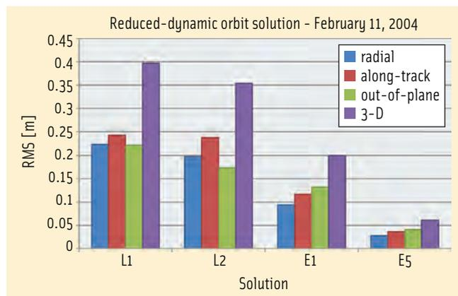
**FIGURE 14** Reduced-dynamic orbit solutions: RMS values (meters) of differences to ENVISAT reference orbit, February 11, 2004
