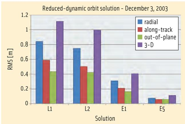
FIGURE 15 Kinematic orbit solutions: RMS values (meters) of differences to ENVISAT reference orbit, December 3, 2003
