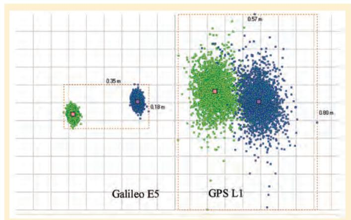
FIGURE 8 Results of the positions comparison for two different periods of observation using single-frequency positioning (after 126 days)
