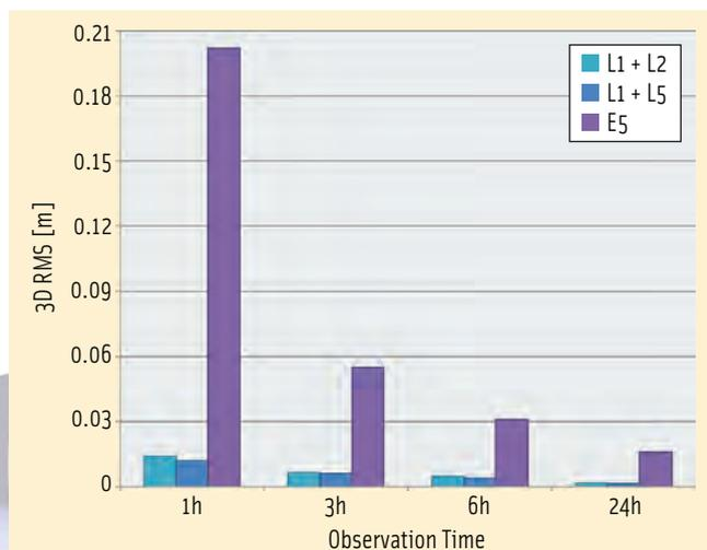
**FIGURE 10** Comparison of the 3D RMS of ionosphere-free combination of carrier phase processing (GPS L1+L2 & L1+L5) with Galileo E5 CPC processing
