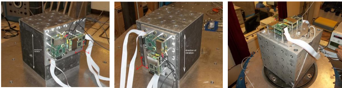
Figure 1: Electrohydraulic and electrodynamic test setups in all three orientations (X, Y and Z respectively).
