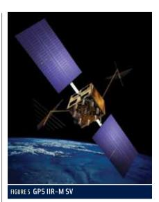
A digital waveform generator will replace the analog boxes creating a fully digital navigation payload capable of generating new navigation signals on-orbit. Lithium-ion batteries will reduce SV weight and provide better EPS performance. Moreover, more M-code power will be added to provide higher power modernized signals to the military.
