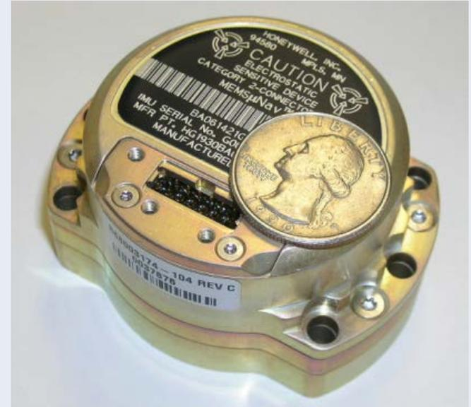
*Honeywell's new flexible low cost, small SWaP, MEMS INS*
