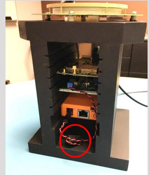
Ferrite chokes put on serial and power cables
