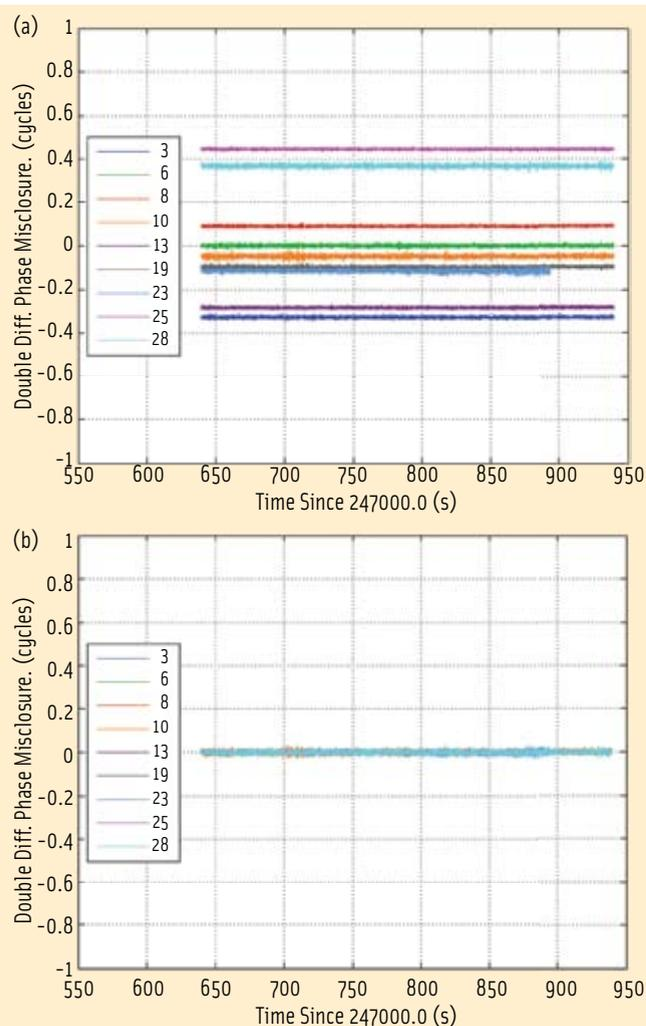
FIGURE 3 Double difference phase misclosures for a zero-baseline test: a) IF phase initialized to 0, b) global IF phase accumulator used.
