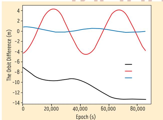
FIGURE 1 Compass MEO-1 orbit prediction errors
