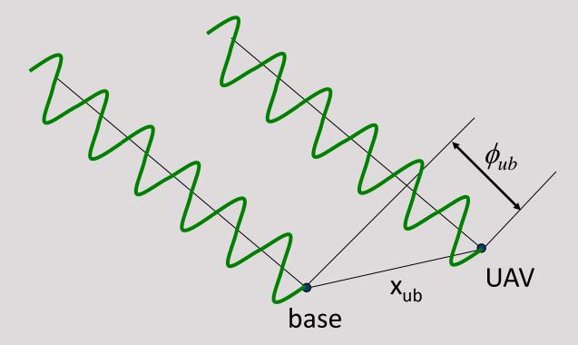
Single Difference removes Iono, Tropo, SV Clock, but adds base clock error
