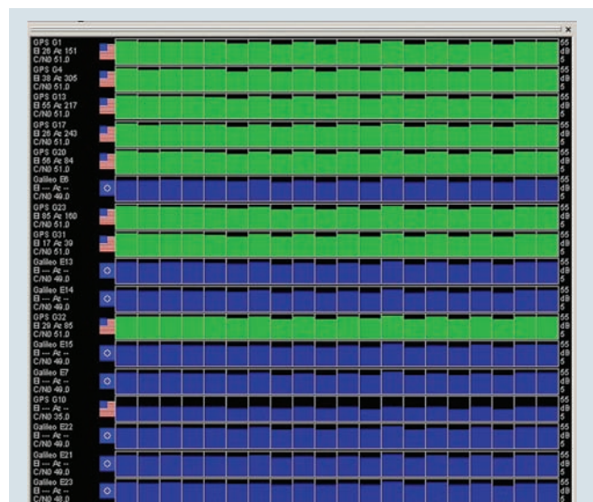
FIGURE 8 Screenshot from the GNSS evaluation software during a systematic interference attack on Galileo E1B. Signals that are tracked are presented in blue, and those for which the navigation message has been recovered are presented in green.
