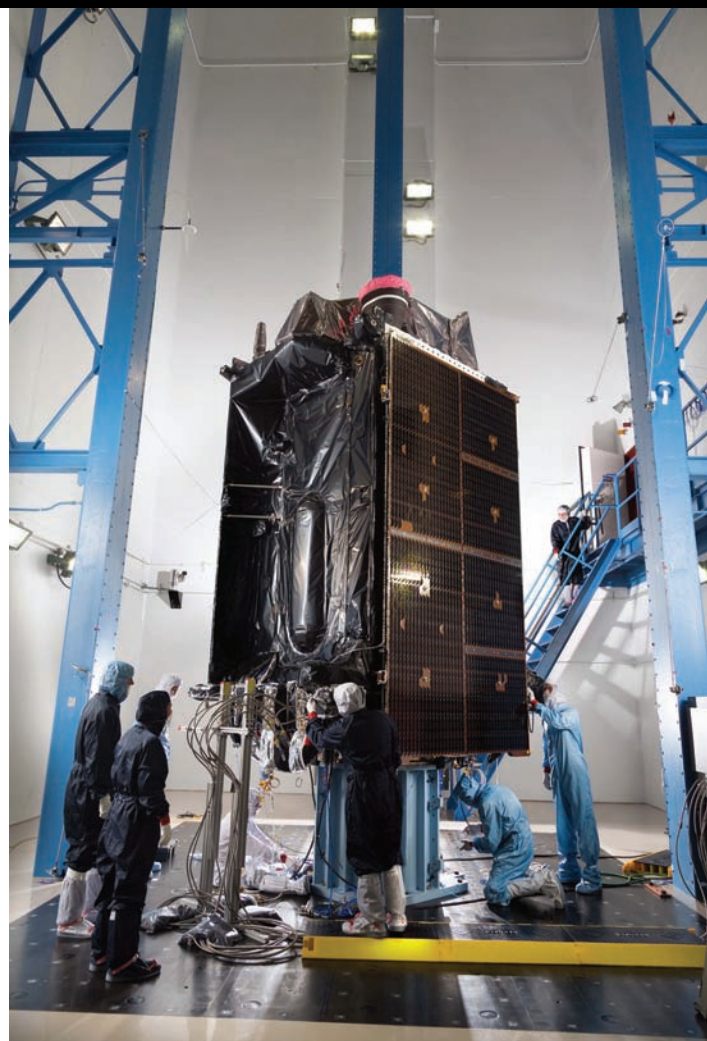
The first GPS III space vehicle has completed acoustics testing, which simulates the launch environment.
