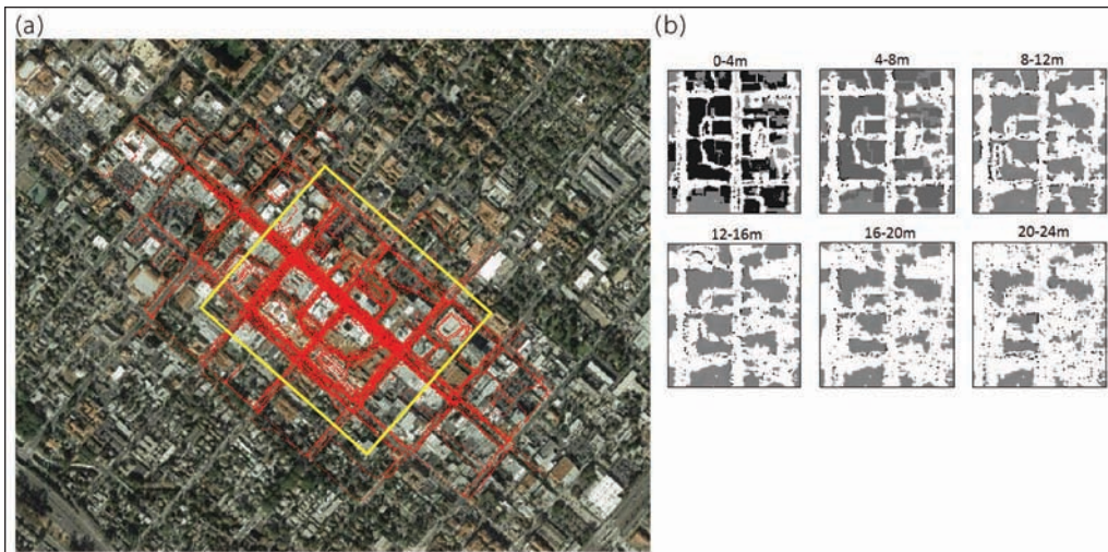
FIGURE 6 Shadow SLAM in downtown Santa Barbara. (a) Mapped area and GNSS traces (b) Horizontal slices of estimated 3D map
