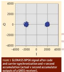
mean squared to the variance of the data in the figure.  $C/N_0$  can be determined once the noise bandwidth of this measurement is known.
