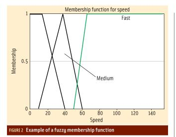
Fuzzy-based AI techniques employ the use of fuzzy set theory, fuzzy operators, and fuzzy inference rules to map input to output. In general, the INS/GPS measurements are *fuzzified* in a step in which the measurements are mapped to a linguistic variable through fuzzy membership functions. An example of a membership function is shown in **Figure 2**.
