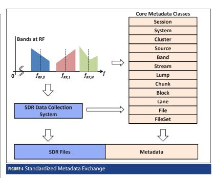
frequency, and the antenna details/ specifications. The metadata standard allows for the specification of a variety of RF bands, each "band" class includes details of the band's center frequency, intermediate frequency, bandwidth and group-delay bias.
