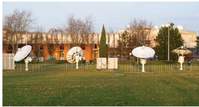
Four dish antennas of a MEOLUT. CNES photo by Emmanuel Grimault, 2014
