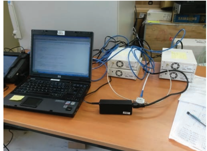
Four USRP digitizers, synchronized on GPS time, sending digitized signal to a laptop
