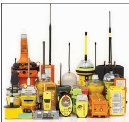
FIGURE 3 Cospas-Sarsat beacons. Image courtesy of Cospas-Sarsat
