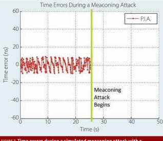
HOURE 7 Time errors during a simulated meaconing attack with a 200-meter separation between the spoofer and the PMU GPS receiver.
