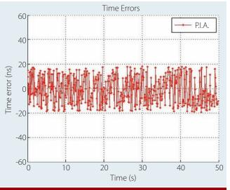
FIGURE 6 Time errors with 9 dB of added noise. Scalar tracking has stopped working.
