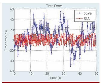
FIGURE 5 Time errors with 4 dB of added noise
