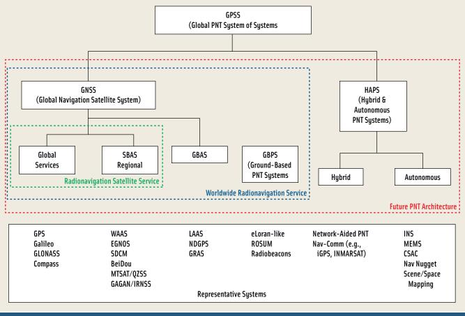
FIGURE 2 The Global PNT System-of-Systems
