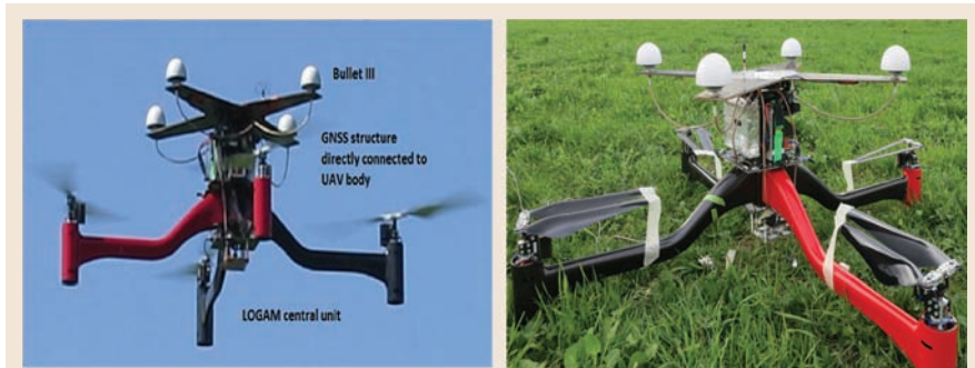
FIGURE 12 The quadrotor UAV where the final system has been mounted. The four GPS antennas are clearly visible
