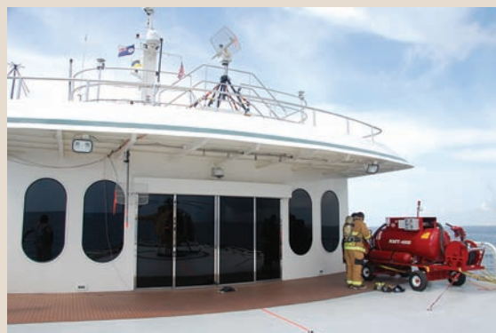
Portable fire suppression system
