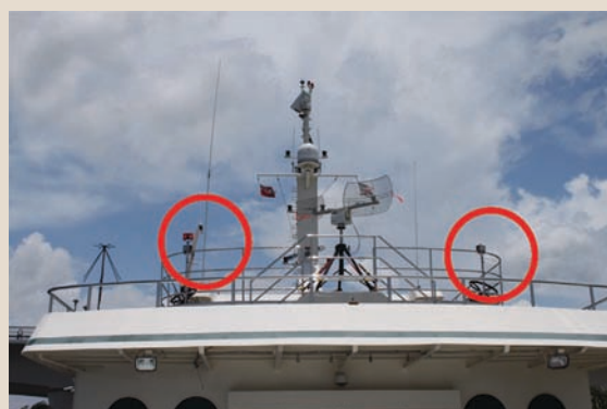
GPS antenna installations
