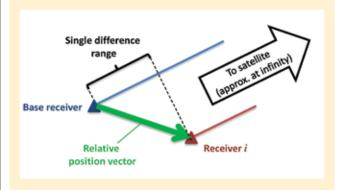
FIGURE 1 Illustration relating single difference measurements to the relative position vector between two points. The single difference measurement is essentially the projection of the relative position vector onto the line of sight vector to the satellite.
