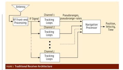
navigation processor (in this case an extended Kalman filter (EKF)) for each signal that is to be tracked. This prediction is performed using the estimated navigation states and the computed satellite position and velocity.
