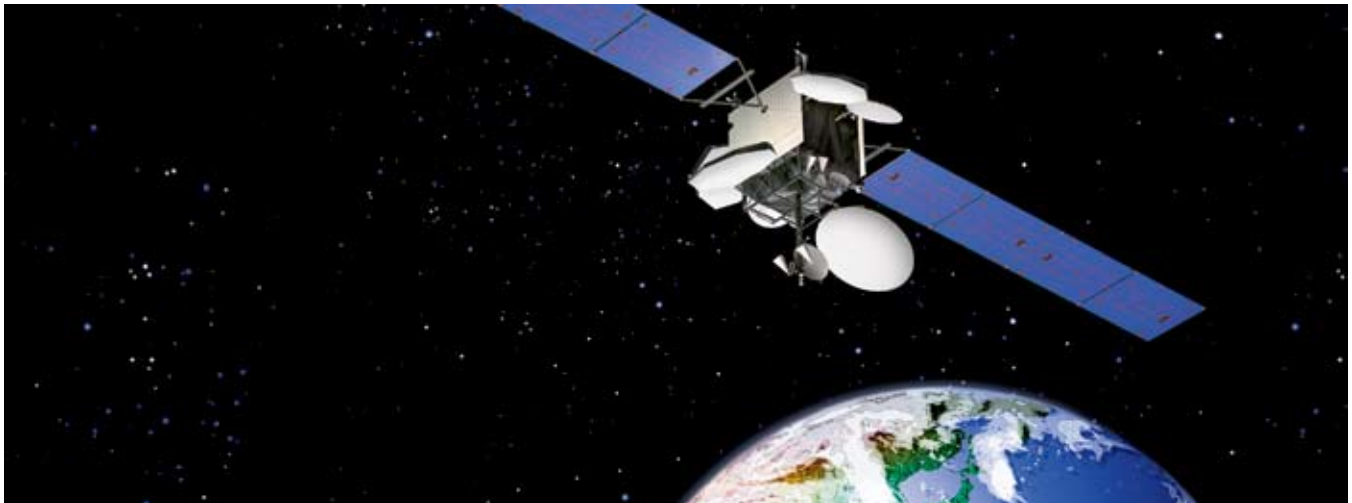
MEASAT-3 satellite with C-band and K-band transponders, The Boeing Company photo
