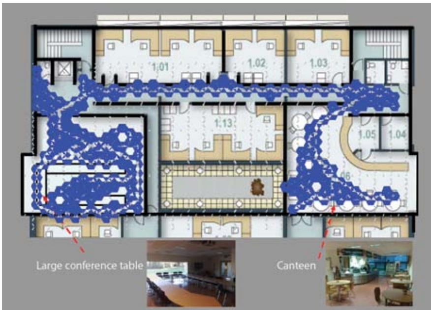
FIGURE 14 A further result of an indoor-only experiment in a different location. The map was generated using 6,000 particles to process 12 minutes of data in faster than real-time on a standard personal computer using a Java implementation.
