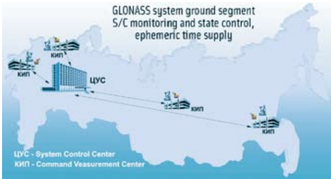
FIGURE 1 GLONASS Ground Control Segment
