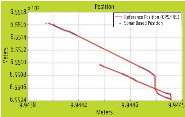
FIGURE 7 XY plot of position – reference and 3-D sonar-based solutions
