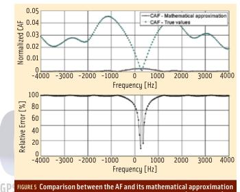
FIGURE 5 Comparison between the AF and its mathematical approximation for a generic value of , i.e.,  $\Delta \tau$ , i.e.,  $\Delta \tau > 1$  chip duration (upper curve); relative error (lower curve)
