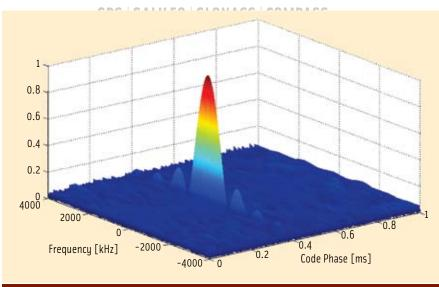
FIGURE 1 Sample of absolute value of AF in absence of noise for the L1 GPS C/A code signal
