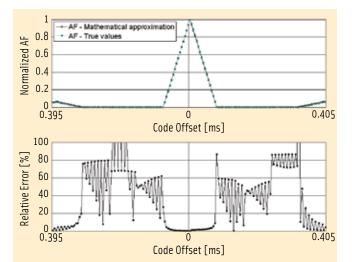
FIGURE 3 Comparison between the AF and its mathematical approximation, given by Eq. (7), for  $\overline{f}_d = f_d$  (upper curve); relative error (lower curve)
