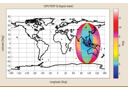
FIGURE 3 Average PDOP value of the six-satellite CAPS constellation over a 24-hour period; white area indicates that the PDOP value is higher than 12.
