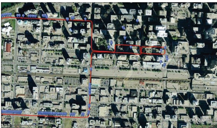
FIGURE 2 Integrated FOG/GNSS trajectory in downtown Calgary
