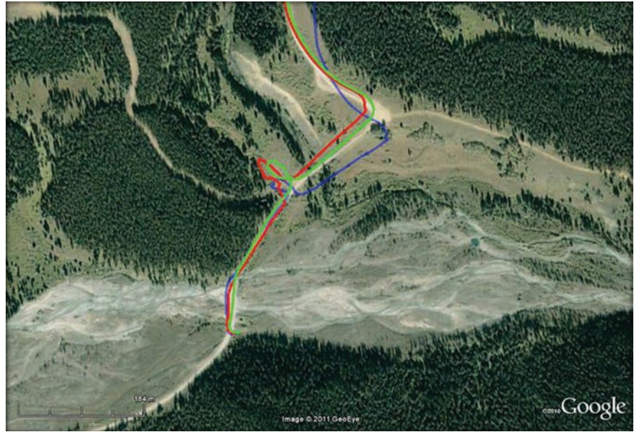
FIGURE 6 Start of the off-road section: reference in green, FOG in red, MEMS in blue
