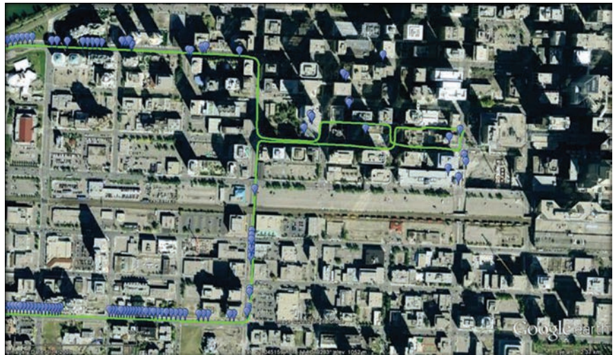
FIGURE 3 Integrated MEMS/GNSS trajectory in downtown Calgary
