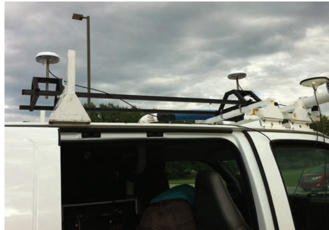
Antenna configurations on trials vehicle: Dual GPS antennas for the INS under test and single GPS antenna for the CIMU
