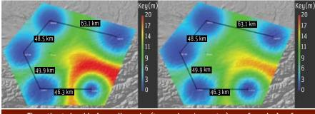
FIGURE 3 The estimated residual non-dispersive (troposphere/geometry) error for a single reference station user (left) and a network reference station user (right).
