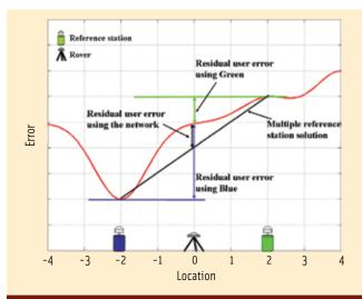
FIGURE 1 Example of the measurement error of one satellite across a region (red line). This error is measured at two locations indicated by the green and blue reference stations.
