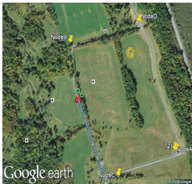
FIGURE 6 Color clustering multiple results for one geolocation (red caution = jammer position, green stars = best solutions, white stars = other solutions). The blue trajectory illustrates the true jammer trajectory.
