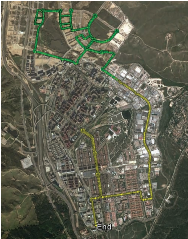
FIGURE 13 Data-Authenticated PVT trajectory from a kinematic test of the Galileo Commercial Service (Tres Cantos, Madrid; green: open sky; yellow: urban – dense urban)
