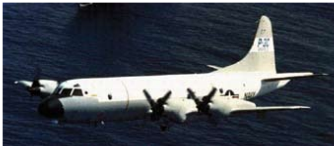
SAASM and GPS RAIM tests were performed on an operational P-3 using SAASM-ISER.
