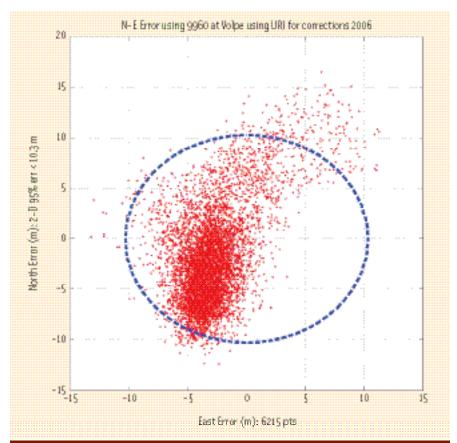
FIGURE 1 Plot of error in the horizontal plane at Volpe National Transportation System Center using University of Rhode Island measurements as corrections (The dotted blue line represents the 95 percent accuracy circle.)
