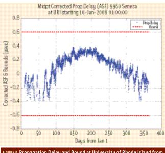
FIGURE 2 Propagation Delay and Bound at Volpe Center from Seneca, New York, transmitter (472 km)
