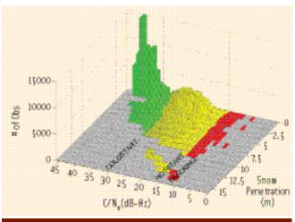
FIGURE 1 Histogram of C/N<sub>0</sub> Measured versus Snow Penetration
