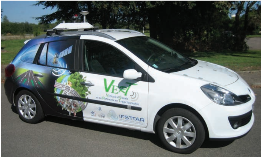
Vehicle dedicated to equipment test and reference trajectory estimation
