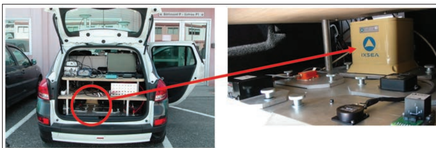
FIGURE 3 Onboard installation of the RTMeS
