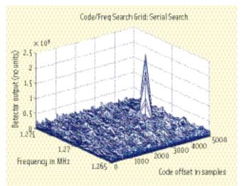
FIGURE 2 Sample Code-Lock Detector Output for a Single Visible Satellite
