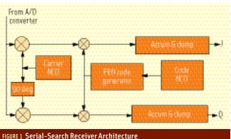
rier and then search through all possible code offsets. If no satellite signal is detected, the frequency setting is changed and the process is repeated. This continues until either a) the satellite signal is acquired, or b) all possible combinations of local code and carrier (known as the search grid) have been searched.
