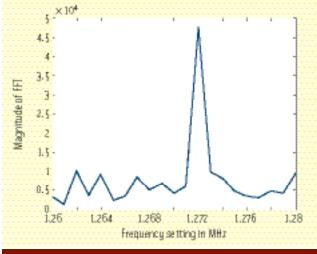
FIGURE 4 Doppler Frequency Determination using Parallel Frequency Search Approach
