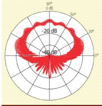
FIGURE 1 Patch Antenna Elevation Gain Pattern (-1 dBiC Peak)
