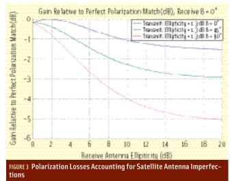
An ideal RHCP antenna would have the same response to any linear polarization stimulus; namely -3 dB relative to its response to an RHCP stimulus. In practice, the antenna gain in two orthogonal polarizations (e.g., horizontal & vertical) is not perfectly balanced. As a result, the antenna will actually have elliptical polarization.
